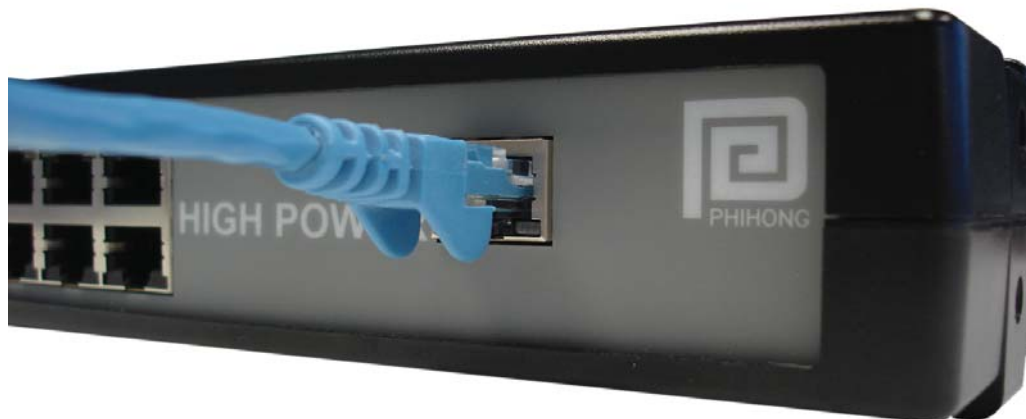
Figure 9: Small Frame Multiport Midpsan SNMP Connection
