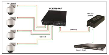
Using standard RJ45 connecting Ethernet cables the POE60S-1AF takes its power from an Ultra or Mega PoE midspan (75W or greater). The output is converted to be IEEE802.3af compatible 15.4W per port. The device can also act as a switchdata repeater by itself. It has an optional 75W DC power adapter, the PSC75U-560 which can power all four ports at 15.4W per port.
