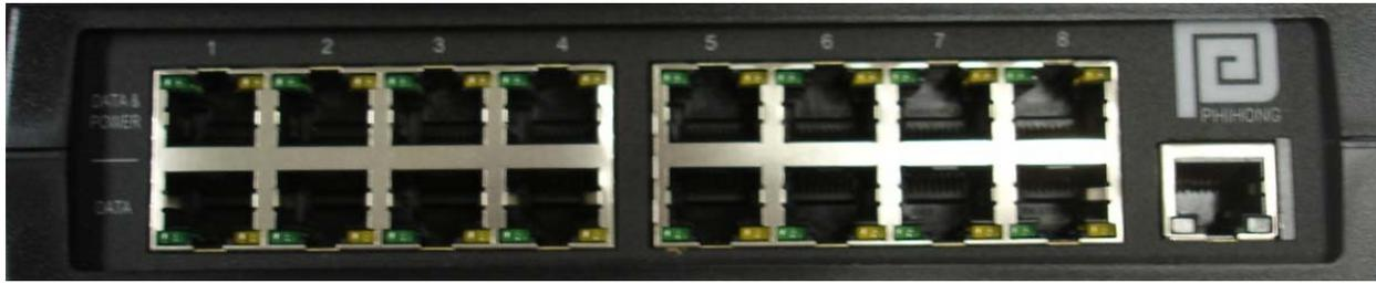
**Fig 1 Front side of Midspan**
