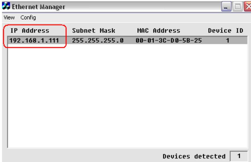
Step 2: Select **Auto Scan**: If a Phihong PoE125U Device is found, the GUI will link to the device automatically.
